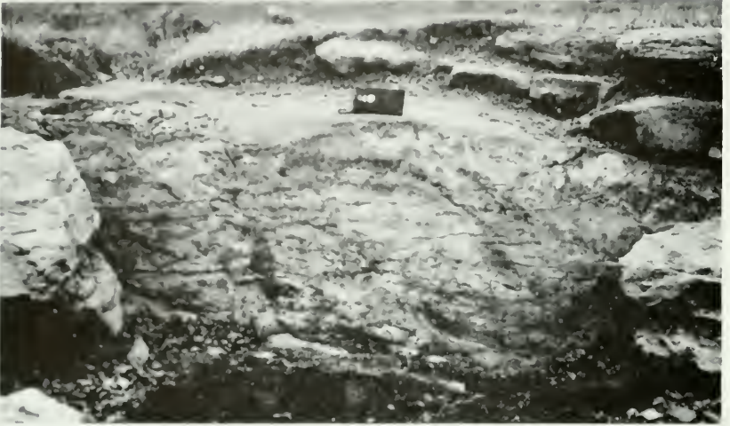
FIGURE A.—Dunite outcrop showing thin overburden and expansion joints paralleling the surface.
